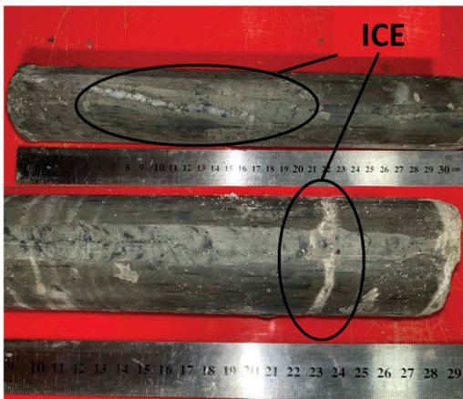
Figure 5. Frozen soil samples with ice lenses collected by direct push sampler mounted on a CPT press at Sharapov Shar.
