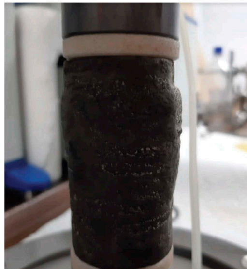
Figure 7. A frozen soil sample after the triaxial test and its failure character.
